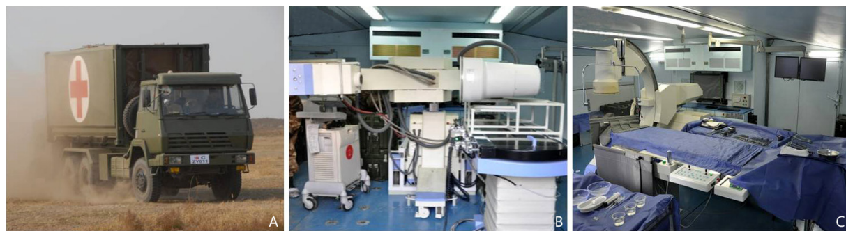
Figure 2. The folded and unfolded states of field intervention cabin. A. Transporting the field intervention cabin; B. The interiors of folded field intervention cabin; C. Working state of the unfolded field intervention cabin
